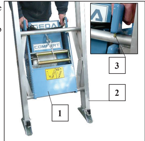
Fig. 31 Using rope winch
